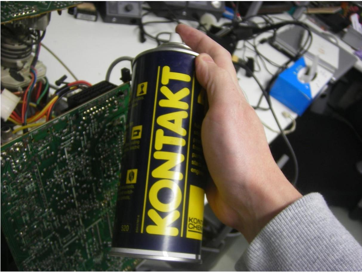
Inject contact spray into all potentiometers.
